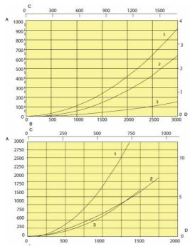
A: Pressure drop, Pa B: Airflow, m3/h C: Airflow cfm D: Pressure drop, in w.c. Top diagram: 1 = Top connection angled, Ø 200 mm 2 = End connection 3 = Exhaust rail, per metre Bottom diagram 1 = Extraction unit LL, hose 4 m, Ø130 mm 2 = Extraction unit LL, hose 4 m, Ø160 mm 3 = Extraction unit HL, hose 2 m, Ø160 mm
